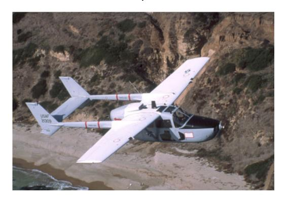
The O-2 is a military version of the Cessna Model 337 Super Skymaster. Distinguished by twin tail booms and tandem-mounted engines, it features a tractor-pusher propeller arrangement. Derived from the Cessna Model 336, the Model 337 went
